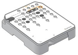
The reagent cartridge includes a designated reservoir for loading prepared libraries. After the run begins, libraries are transferred automatically from the reservoir to the flow cell.
