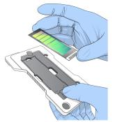
3 Using the openings on either side of the BeadChip, make sure that the BeadChip is seated in the recessed shelf of the adapter.
