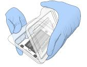
4 Clean the glass surface of the flow cell with a lint-free alcohol wipe. Dry the glass with a low-lint lab tissue.
