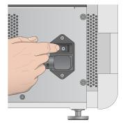
1 Press the power button above the reagent compartment. The power button turns on the instrument power and starts the integrated instrument computer and software.
