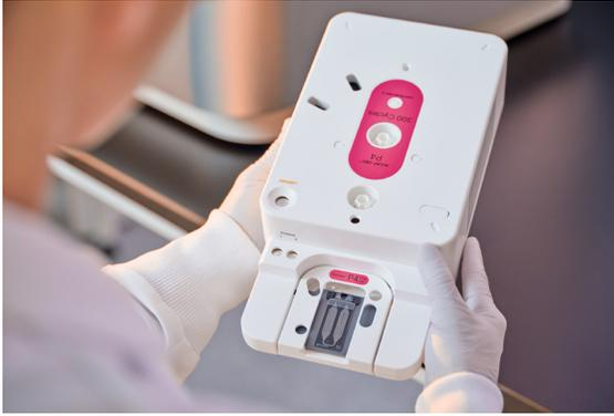
The integrated cartridge includes reagents, fluidics, and the waste holder. Simply thaw and prepare the reagent cartridge, insert the flow cell, load the library, and place into the instrument.
